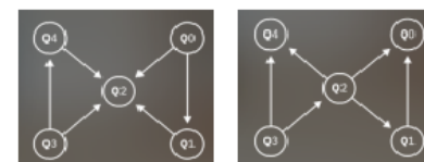
Figure 1. Diagram of the available cNOTs among qubits on the IBM 5Q computers: ibmqx2 (left) and ibmqx4 (right). The qubits are represented by circles, while the cNOTs are arrows pointing from control qubit to target qubit.
