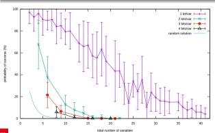
Results on DW-2000Q (the resolution on the couplers' setting is limited to about  $10^{-3}$ )
