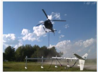
Eagle Geophysics' Multi sensor Gradiometer, measures 10 vertical G horizontal gradients.
