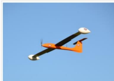
Development of the MOIARCH fixed wing Gradiometer was based on GEM's re-designed, Ultra Light Weight Potassium technology sensors. Now, GEM's DRONEmag™ sensors have become standard across all UAV magnetometer platforms.
