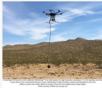
A magnetometer can be flown with a fixed-wing aircraft or a drone system for high resolution surveying at 10 m line spacing, maximum 300m across their conventional and new surveying. DRONEmag™ is high resolution to detect the subtle variations due to the ability to resolve near subtle signals at standard 100-foot above magnetometer flying heights. Photo courtesy of BRGM.com/brgm.com
