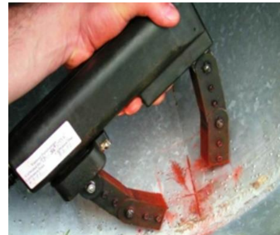
Magnetic particle – Breaking surface flaw image
