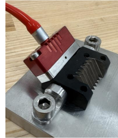
Phased array probe (350 °C)
