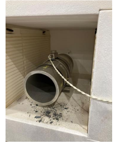
Thickness monitor in box oven (400 °C)
