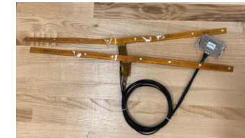
Sensors in flex circuit (180 °C)
