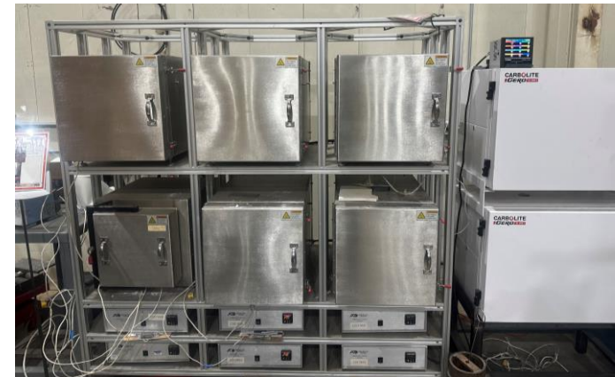
Box furnace battery (1200 °C)
