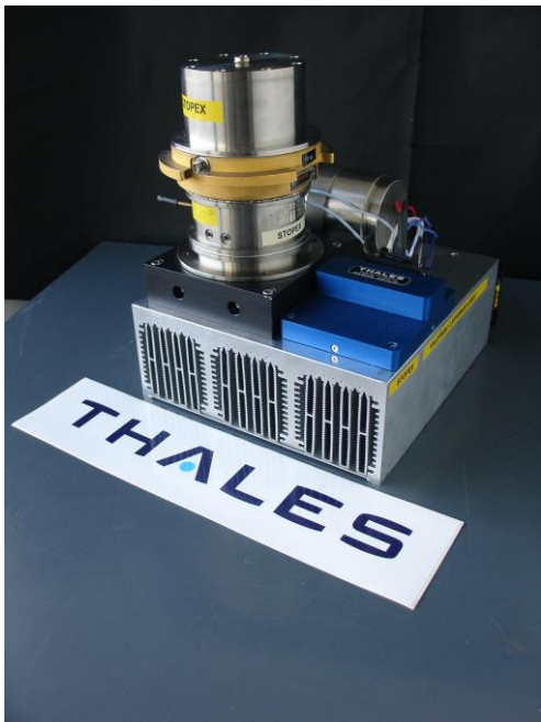
Superconductor based mux/demux and filters in a compact cryocooler for naval applications
