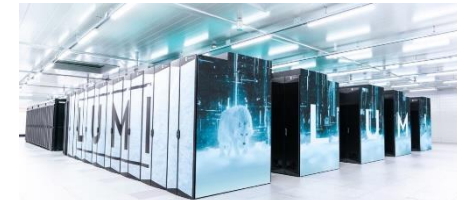
# 5, LUMI-G (EuroHPC), ~380 PF HPL, 2023, 7 MW, CSC, Finland, HPE Cray, ~10K AMD MI250X
