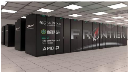
# 1, Frontier, 1.2 EF HPL, 2022, 22MW, Oak Ridge National Laboratory (ORNL) HPE Cray, ~38K AMD MI250X
