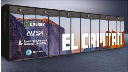
El Capitan, >2 EF peak, Q1/2024, ~30 MW, Lawrence Livermore National Lab HPE Cray, AMD MI300A APU
