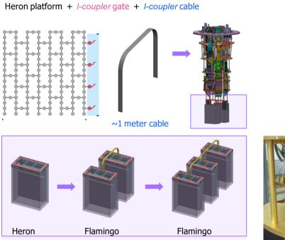
L-coupler demonstrated in 2023 with internal quality factor exceeding the required 95% state transfer fidelity.
