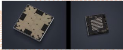
Computing: Superconducting qubits and parametric amplifier (for control and readout of qubits)
