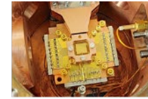
Computing/Sensing: (Left) Trapped ions Paul trap , (Right) Chip ion trap
