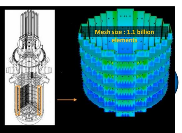
Thermal Analysis of core internal struture bolt in a Nuclear Power Plant
